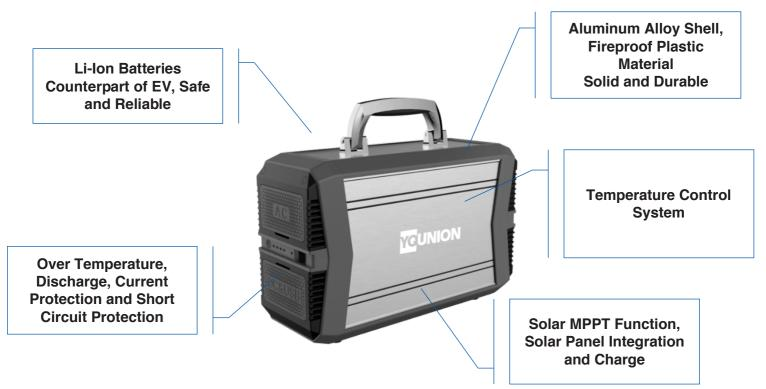
Battery type: 18650 batteries USB1 output: 5V/3A DC output: 12V/8A (MAX) AC output: 220V/300W/50Hz, 110V/300W/60Hz Input voltage: 15V-30V Input current: 5A (MAX) Battery capacity: **11.1V 31.2Ah** Charging time: **5.5-7 hours** Static power consumption:  $\leq$ 200uA Cycle life:  $\geq$ 800 times (capacity  $\geq$ 80%) Working temperature: -10°C---65°C Volume: 300\*117\*208MM Weight: **5.0 kg**
