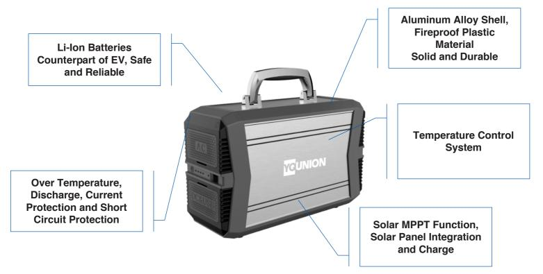
Battery type: 18650 batteries USB1 output: 5V/3A USB2 output: 5V-3A/ 9V-2A/ 12V-1.5A DC1--DC4 output: 12V/8A (MAX) DC5 output: 19V-3.5A (MAX) AC output: 220V/500W/50Hz, 110V/500W/60Hz Input voltage: 18.5V-30V Input current: 10A (MAX) Battery capacity: **14.8V 49.5Ah** Charging time: **6.5-8 hours** Static power consumption:  $\leq$ 200uA Cycle life:  $\geq$ 500 times Working temperature: -10°C---65°C Volume: 381\*128\*243MM Weight: **7.9 kg**
