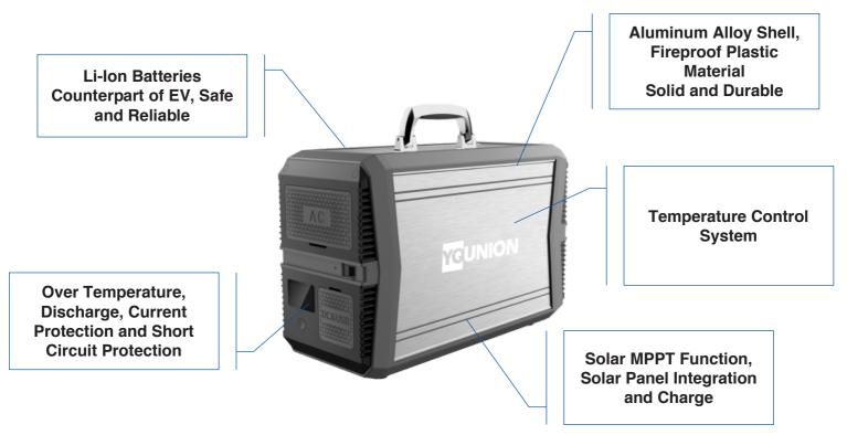
Battery type: 18650 USB1 output: 5V/3A DC output: 12V/8A (MAX) AC output: 220V/1000W/50Hz, 110V/1000W/60Hz Input voltage: 32V-45V Input current: 8.0A (MAX) Battery capacity: 25.9V 39Ah Charging time: 5.5-7 hours Static power consumption:  $\leq$ 200uA Cycle life:  $\geq$ 800 times (capacity  $\geq$ 80%) Working temperature: -10°C---65°C Volume: 408\*163\*256MM Weight: 11.5 kg
