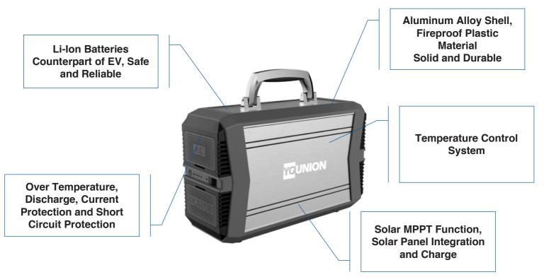
Battery type: 18650 batteries USB1 output: 5V/3A USB2 output: 5V-3A/ 9V-2A/ 12V-1.5A DC1--DC4 output: 12V/8A (MAX) DC5 output: 19V-3.5A (MAX) AC output: 220V/500W/50Hz, 210V/500W/60Hz Input voltage: 18.5V-30V Input current: 10A (MAX) Battery capacity: 14.8V 36Ah Charging time: 5.5-7 hours Static power consumption:  $\leq$ 200uA Cycle life:  $\geq$ 800 times Working temperature: -10°C---65°C Volume: 381\*128\*243\*MM Weight: 7.5 kg
